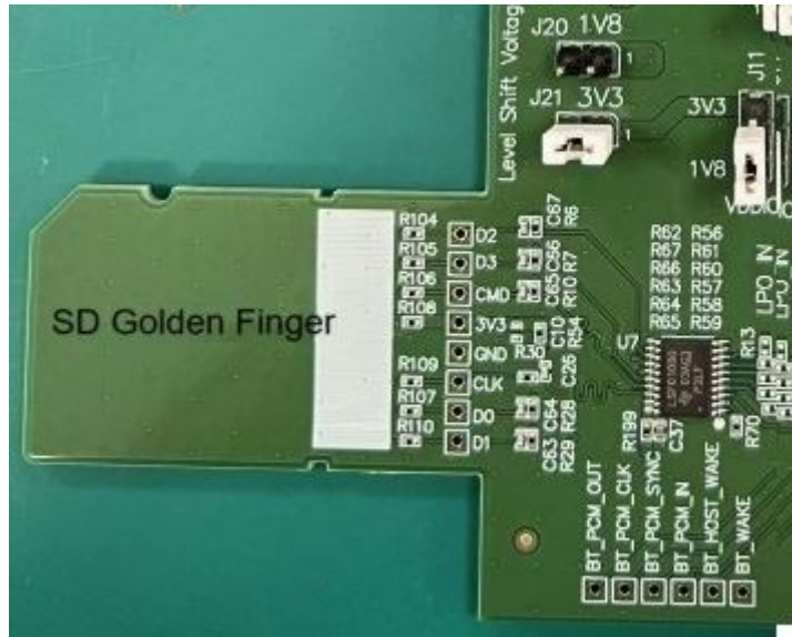
Figure4. EVB interface to HOST SDIO 3.0.
